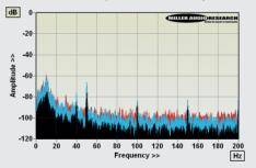
ABOVE: Unweighted bearing rumble from DC-200Hz (black infill) versus silent LP groove (with vacuum pull down, blue; without, red) re. 1kHz at 5cm/sec
