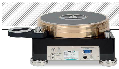
**ABOVE:** As with all TechDAS decks, pneumatic hoses from an outboard pump [see below] are connected to air-bearing 'Flotation' and LP hold-down 'Vacuum' fittings while power, pump and speed controls are communicated via a multi-pin connector
